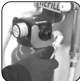
The connecting pipes are delivered bent, but may have been bent to an unsuitable shape during transport.
