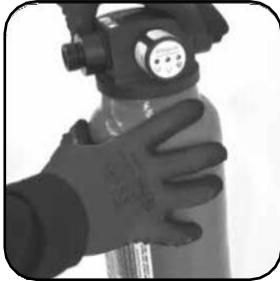
Unscrew the connection head from the cartridge and pull it upwards.
