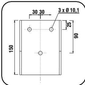
Select an easily accessible location for wall mounting of the stainless steel connection fitting. The masonry to which the water filter system is to be installed must have sufficient strength and load capacity of at least 20 kg. We do not recommend mounting the station on walls with old sanding plasters.
