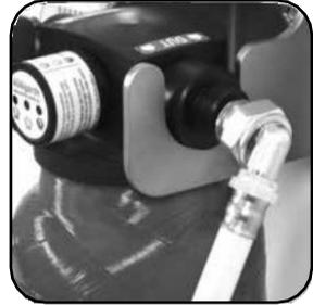
Loosen the screw connection. Unhook cartridge.
